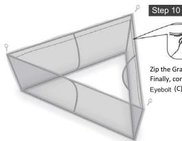
Zip the Graphic closed all the way around. Finally, connect the wirerope (F) to the loops of Eyebolt (C).
